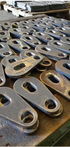
Source Metals provides quality flame cutting as a metal cutting service with quick turnaround times. Our flame cutting department uses Messer CNC controlled machines that provide accuracy as well as speed. Partnered with operators fully equipped with tools and training needed to achieve close tolerance and quality burnouts.
